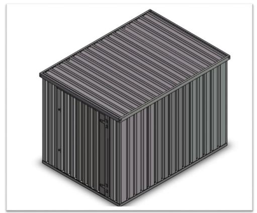
12. Roof is fixed with bolts from connection points inside of the store.
